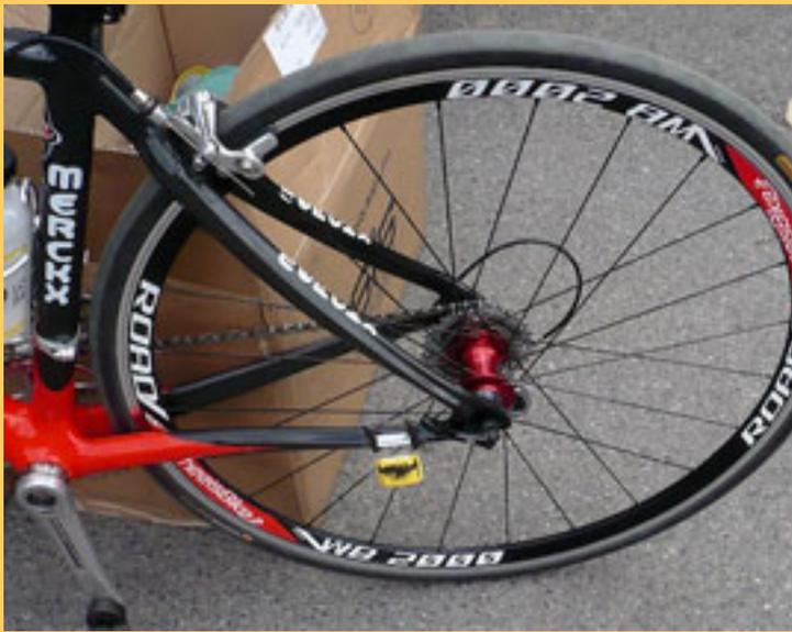
anyhoo, the back end eschews the smooth roundness of the main part of the frame and becomes angular along the length of the stays (really awkward to fit a transponder, if truth be known) though i did like the way the chainstays curved outwards towards the dropouts.
